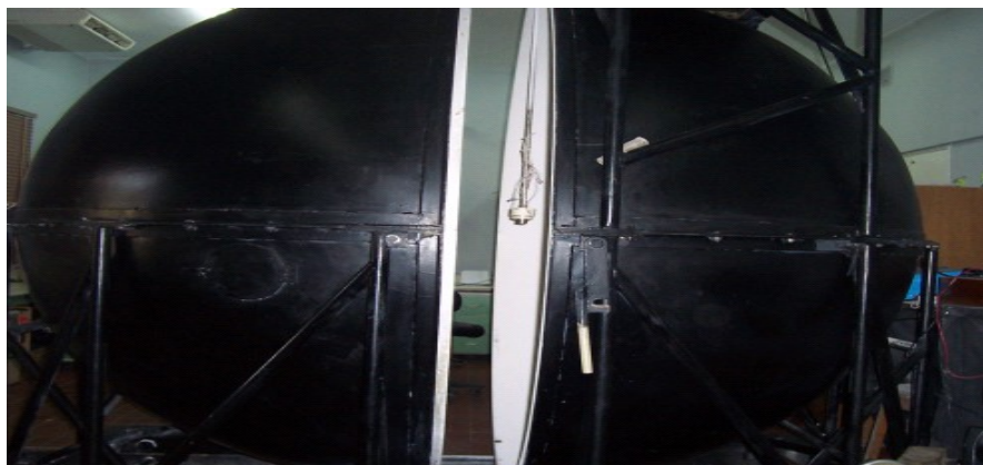
Figure.2 The Lamp baffle, the photometer port, and the lamp holder of the 2.5 integrating sphere system
